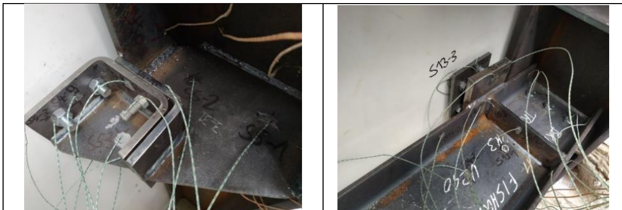
Figure 3.4: View of the tested fusible systems inside the furnace
