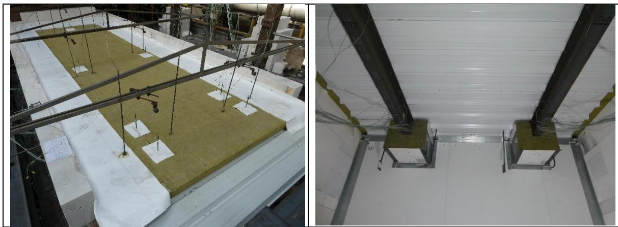
Figure 4.3: view of the test specimen after assembly (outside and inside the furnace)
