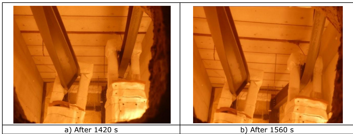
Figure 3.13: Deformed shape of semi-portal frames during the test
